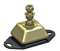
IM-Mountings are very suitable for mobile applications. These compact antivibration mountings are easy to install and offer a high level of vibration insulation. The integrated rebound control-device limits excessive movement under shock loads. IM-Mountings are available in several rubber mixes to accommodate a large load range. These mountings can be supplied with a height adjustment feature.
